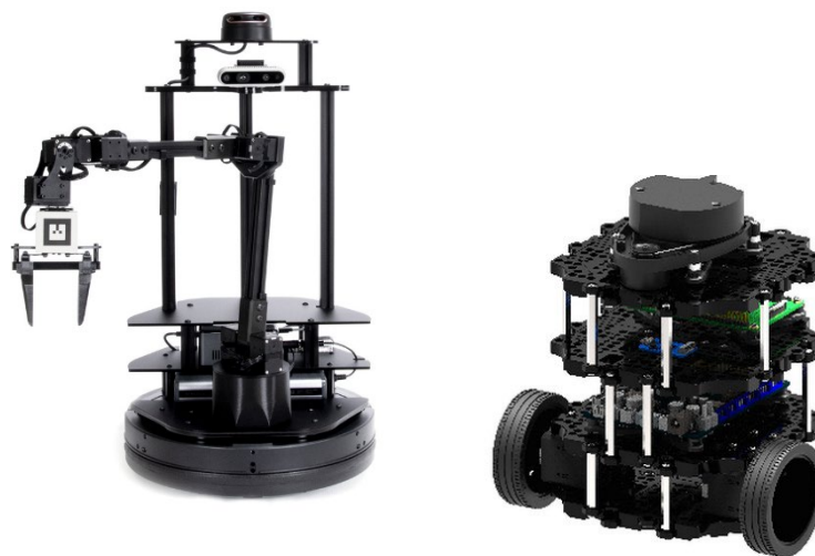
Figure 1. On the left: LoCoBot WX250 6DOF. On the right: Turtlebot3 Burger
