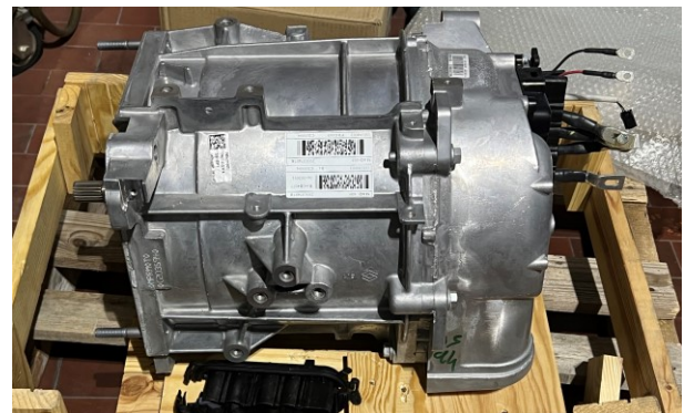
Fig. 2. View of the EESM adopted by Renault Zoe R135 and used for the experimental validation.
