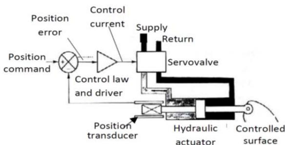
Fig. 1: Concept schematic of the EHA actuator
