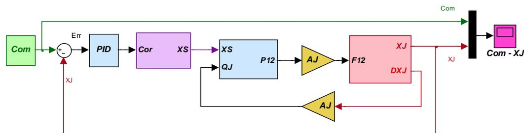
Fig. 2: Simulink block diagram of the considered EHA.
